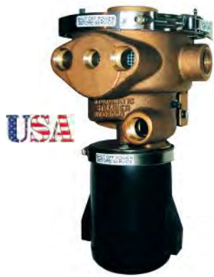
970-1500 Provides filtered water to multiple devices, and has a 1-1/2" NPT inlet port with multiple 1/2", 3/4" and 1" ports for connecting devices. Debris is pumped out through a 3/4" NPT port.
